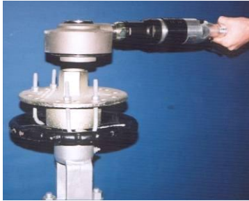
Valve is closed, KMS is placed on top of adaptor
