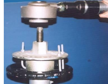
Valve is open, remove KMS handheld actuator
